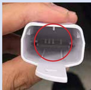
**Figure 2.1:** Deformed contact sheet inside the sensor
