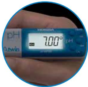
Monochrome digital display with switchable backlight
