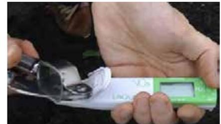
**Figure 4:** Placing sap directly onto LAQUATwin nitrate sensor.
