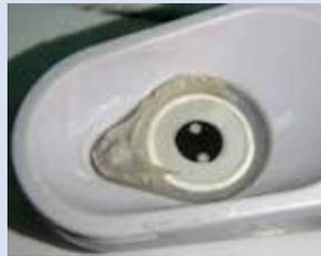
**Figure 1.1:** KCl salts build-up on the sensors is a normal occurrence
