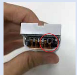
**Figure 3.1:** Bent pins inside the meter
