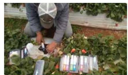
**Figure 6:** Irrigation water testing with LAQUATwin pocket meters.
