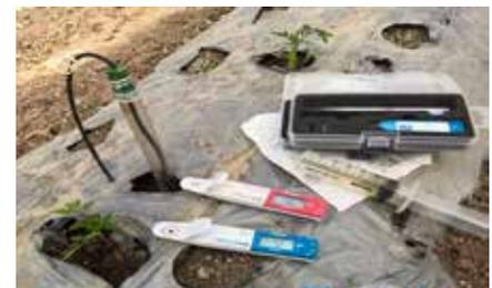
**Figure 5:** pH and conductivity testing on soil solution.
