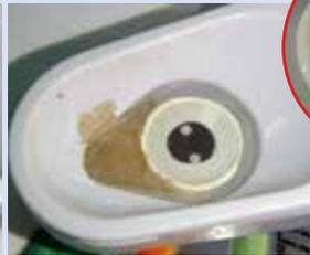
**Figure 1.2:** Sensor with cracked or broken membrane
