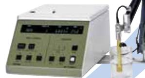
Model F-80 (benchtop) The world's first instrument capable of measuring pH at 0.001 resolution includes an integral computer with automatic calibration and a self-diagnostic function.
